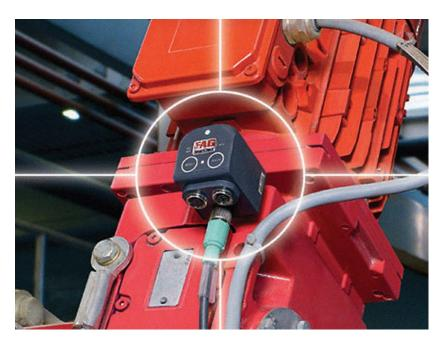
Easy mounting of the SmartCheck sensor unit with a screw on top of the motor or gear box and connecting with a single cable due to Power over Ethernet (PoE) technology
